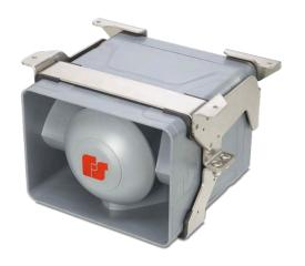
Model eHorn-HV is an electronic horn capable of producing two high decibel horn tone outputs from the same unit through internal amplification and tone circuitry. The eHorn-HV's potted internal electronics and external heavy-duty mounting bracket allow the unit to withstand high-vibration environments.
