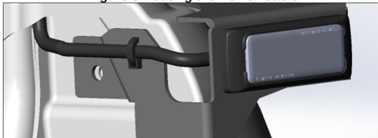
Figure 3 Routing the Power Cable
