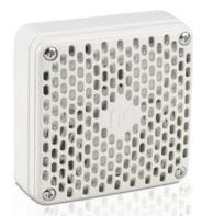
Model 450E electronic horn offers a loud, clear and distinctive tone. It's often used for general alarming, start and dismissal noticing, coded paging and process control in noisy areas. Its 4-wire terminal block and supervisory diodes design make it ideal for fire alarm applications.
