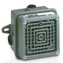
Model 350WB Vibratone<sup>®</sup> Horn produces a loud tone by the electro-mechanical vibration of the diaphragm. The horn mechanism with diaphragm is attached to the grille. Indoor or outdoor use is made possible by the water- and dust-tight back box.
