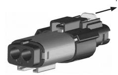
**2.** Fully press the locking latch. To allow the connectors to be separated, the locking latch must be fully depressed to release the locking ramp on the plug.
