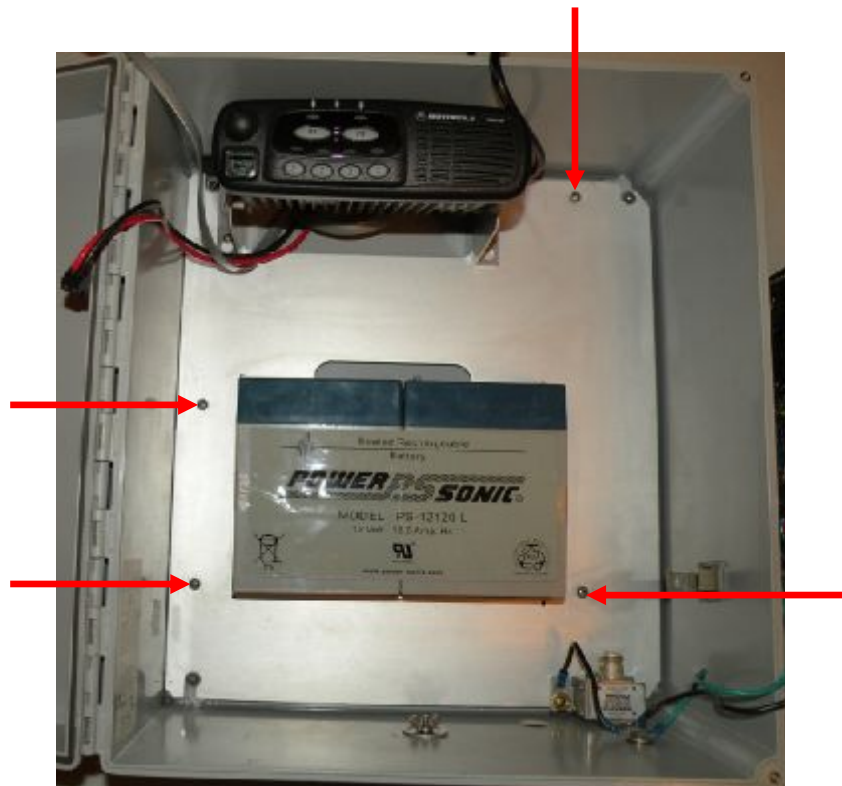
Figure 9.2 - UVRI Battery Location and Cover Plate Mounting Screws
