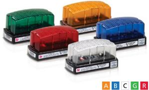
Model LP1 low profile strobe light is a rectangular Type 4X strobe light that is available in five colors: Amber, Blue, Clear, Green and Red. The LP1 is designed to be flush mounted to control panels or other flat surfaces. Mounting is accomplished with two supplied 1-1/4" 8/32 slotted hex bolts. A neoproene gasket is supplied to create a water-tight and dust-tight seal. The gasket mounts between the base of the light and the mounting surface.
