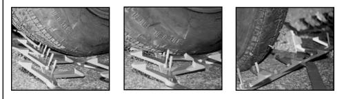
Typically, a tire picks up between four to six spikes and deflates in 12-20 seconds.
