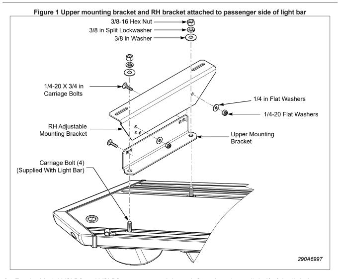
**4.** For the Model VSLR6 and VSLR8, repeat steps 1 through 3 on the other split half of the light bar.
