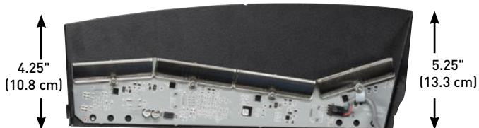
SIFZJ models* Reflector layout for Advanced Off-Axis
