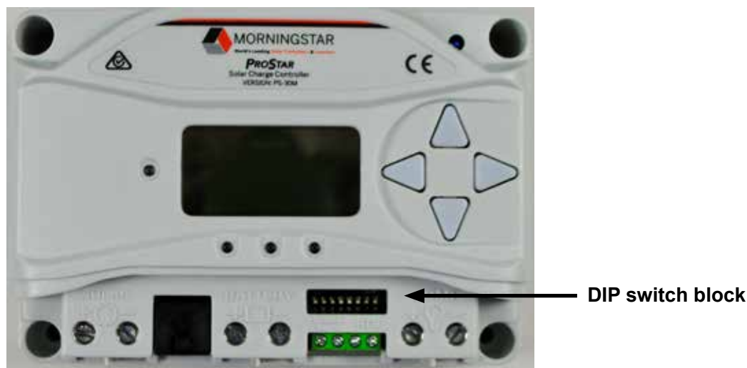
Figure 11 PS-30M Solar Regulator
