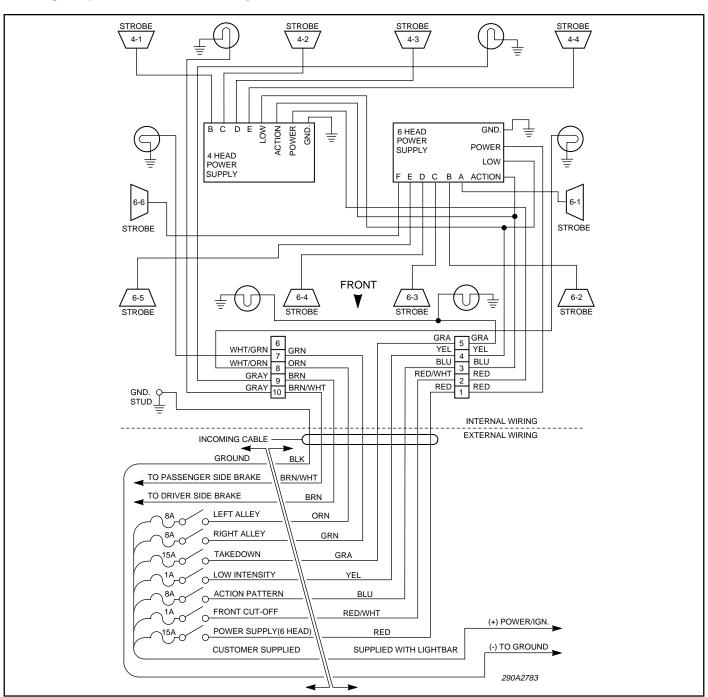
Figure 1. SJL3P-CPD Wiring Diagram.
