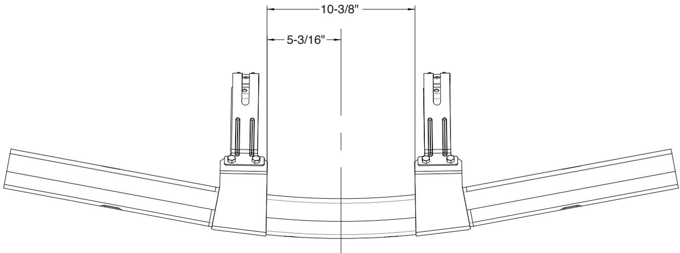
**Figure 4** Speakers installed on bumper with logos facing center of vehicle
