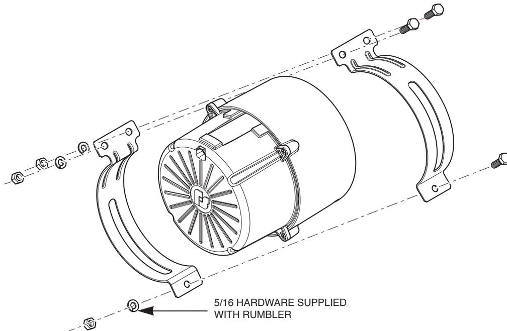
6. Secure the speaker in the bands with the 5/16" hardware supplied with it.
