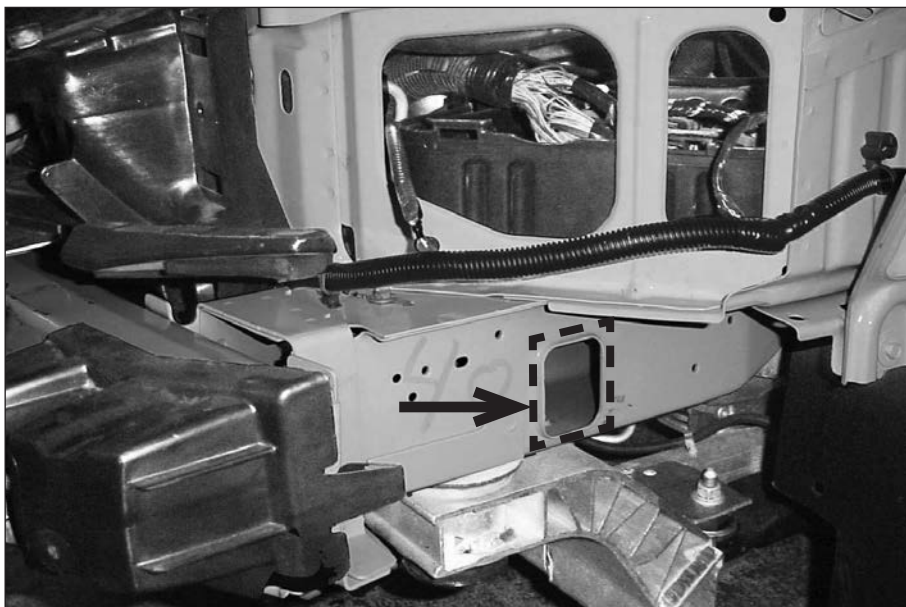
Figure 1 Area used for mounting the speaker (bumper removed for clarity)
