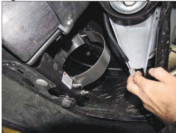
Figure 4 Bands attached to Rumbler® mounting bracket
