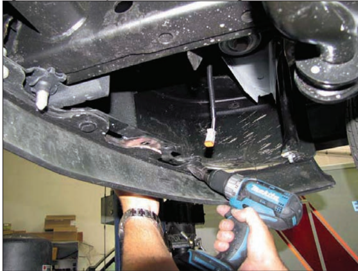
Figure 2 Hole for plastic fastener enlarged with core drill bit
