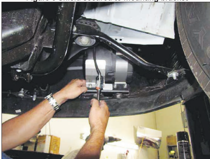
Figure 6 Shield secured to mounting bracket
