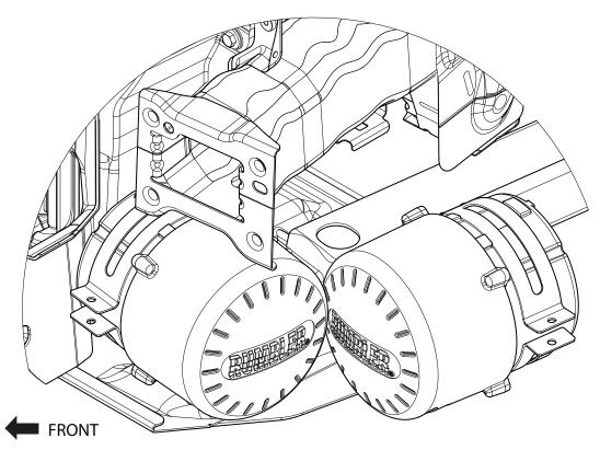
Figure 5 Orientation of forward and rearward speakers
