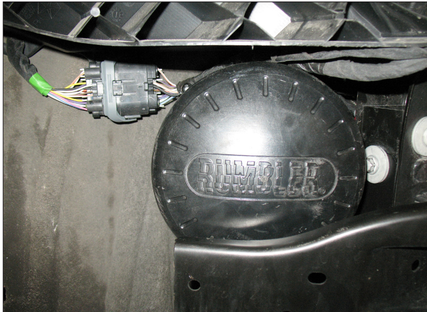
Figure 6 Driver-side Rumbler installed
