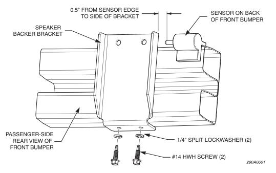
Figure 3 Backer bracket attached to passenger-side bumper
