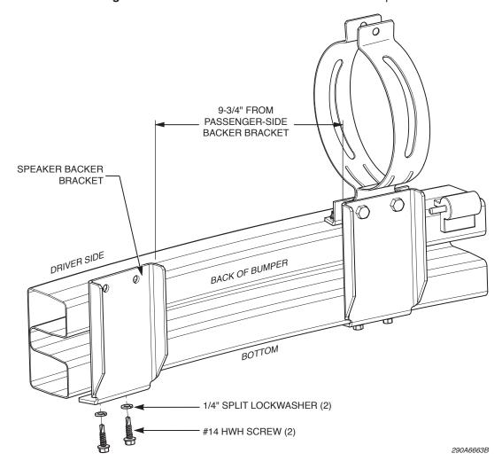
Figure 5 Driver-side backer bracket attached to bumper
