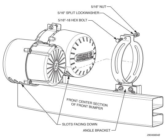
Figure 6 Driver-side backer bracket attached to bumper
