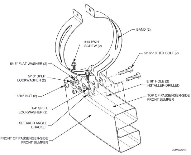
Figure 4 Bands attached to bracket
