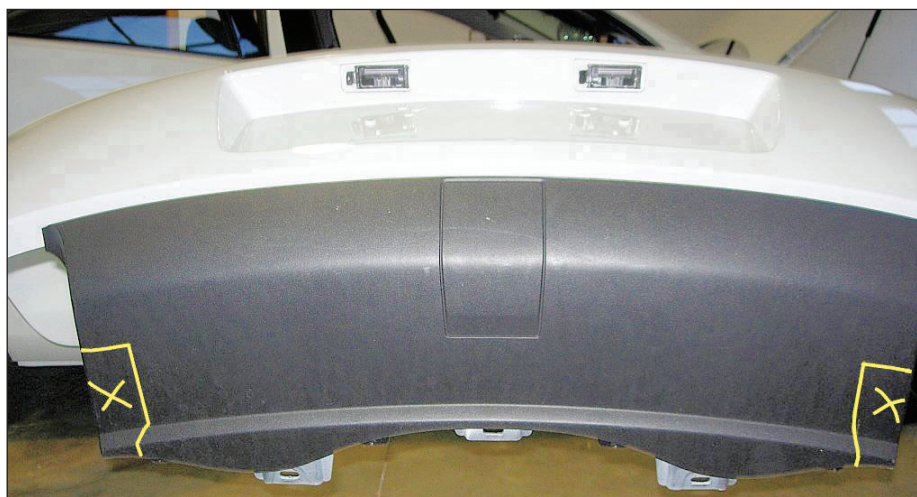
Figure 4 Two 3" x 6" sections marked in lower splash panel
