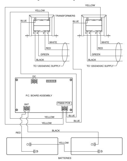
Figure 4 PS600 Wiring schematic
