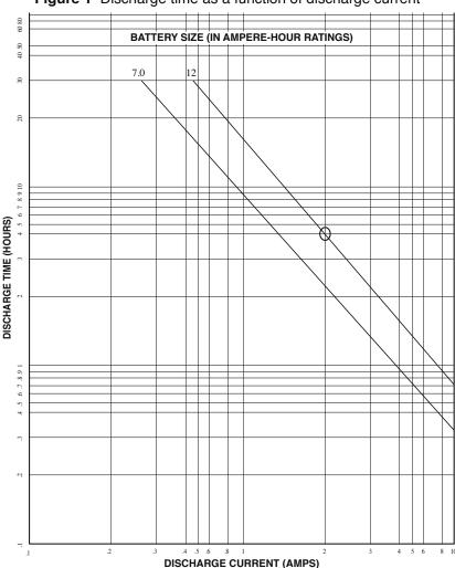
Figure 1 Discharge time as a function of discharge current
