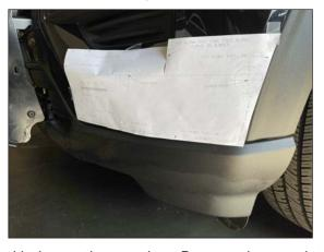
**6.** Using a center punch, mark the center of the two specified holes on the template. Remove the template; using a 1.5-inch hole saw, cut out the two holes and then clean the edges. See Figure 7. Repeat this process on the passenger side.
