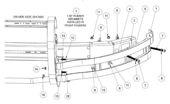
3. See Figure 1. On one side at a time, attach the inner mounting brackets for the pit bar (Item 2) to the steel bumper channel using the supplied long M10 hex bolts (Item 9), cupped washers (Item 10) and flange nuts (Item 11) (use the yellow zinc plated hardware) (Figure 3.)
