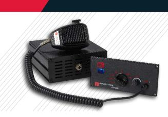
The PA4000 is a full-featured, programmable, electronic siren and light control system with a remote-control head that can be flush mounted to any flat surface. The design of the PA4000 siren system is ideal for use in ambulances, police cars, fire apparatus and command vehicles.
