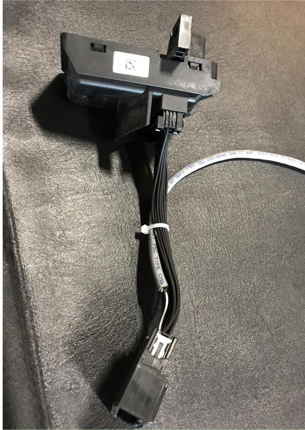
4. Plug the other end of the OBDCABLE6-2 or OBDCABLE25-2 into the Pathfinder. Refer to the Pathfinder Installation Manual.
