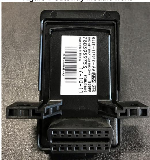
2. Unplug the 24-pin connector from the Gateway Module, and then plug in the Federal Signal OBDCABLE6-3 or OBDCABLE25-3.
