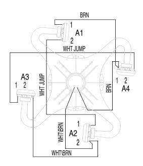
TOP VIEW FIRST ACTIVE MODULE DRIVER ORIENTATION
