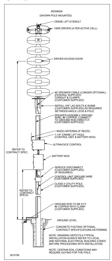
Figure 3 Typical Wooden Pole-mounted Installation
