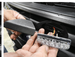
MicroPulse C Series shown with optional stud mount for easy installation
