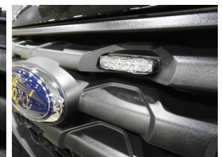
MicroPulse C Series shown mounted in grille
