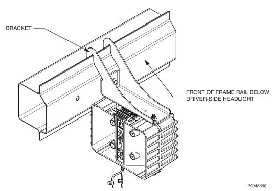
Figure 2 AS124 speaker installed on frame rail with bracket
