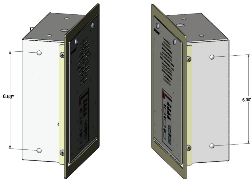
Figure 4 Side View - Hole Measurements
