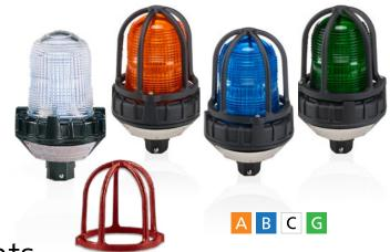
These models are hazardous location strobe lights that provide 60 high-intensity flashes per minute. This warning light is available in 24VDC with a 4-wire supervisable power circuit for fire alarm and suppression supervised control panels.
