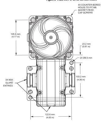
Figure 3 Front view of Ex de surface mount
