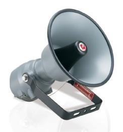
SSTX3-MV is an explosion-proof electronic siren capable of producing three high decibel tones from the same unit. The integrated circuitry is contained in a rugged die-cast aluminum housing. The unique threaded rear access cover eliminates traditional time consuming bolting patterns. The access cover is also equipped with a braided cable lanyard securing it to the housing whenever the cover is open for installation or maintenance.
