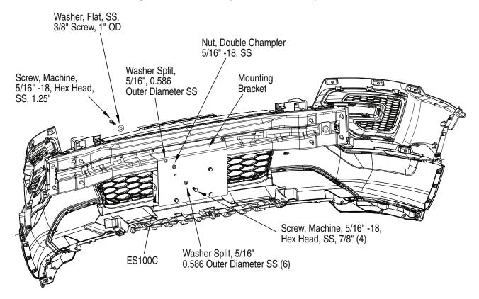
Figure 1 Back of bumper with ES100C Speakers
