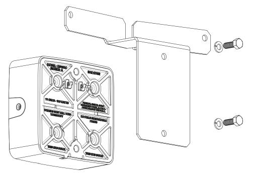
Figure 2 Mount the speaker to the bracket
