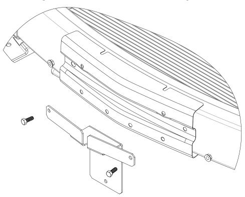
2. See Figure 1. Position the bracket over the existing holes as shown and secure with the 5/16 bolts and flanged nuts in this kit.
