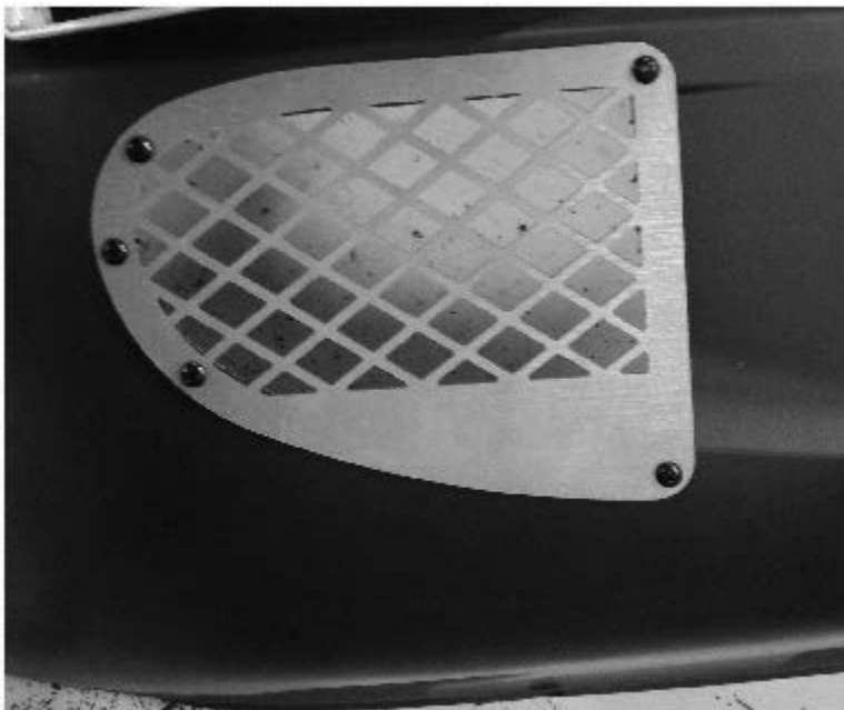
Figure 3 Grille mounted on passenger-side front fascia
