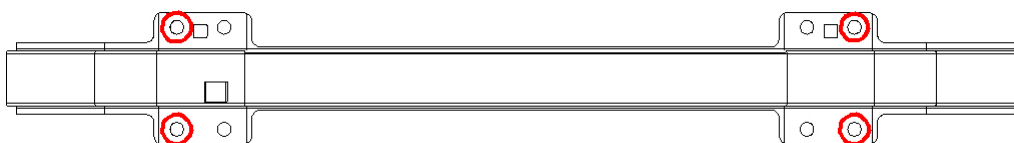
Figure 2 Remove the bolts
