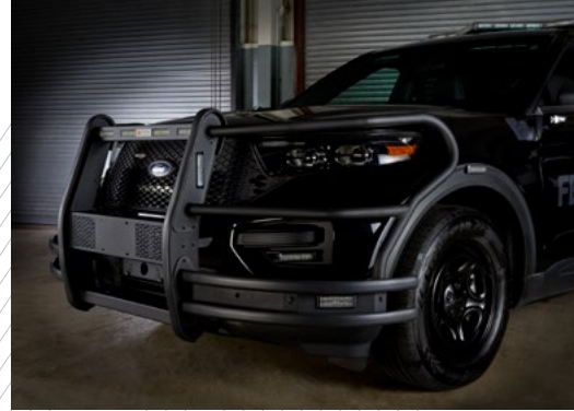
Push Bumper, Top Channel, Lower Guard and Upper Guard shown installed on a Ford Police Interceptor Utility
