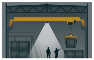
371LEDX with the 371LED-KIT-CR reflector installed reflects the light beam at 22.5 degrees from the vertical orientation resulting in a focused light output.
