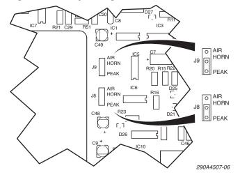
Figure 5 Horn Configuration - Air Horn
