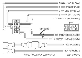
To allow incoming radio messages to be rebroadcast over the outside speakers, connect the two brown zip cord leads (pins 1 and 2) across the two-way radio's speaker.
