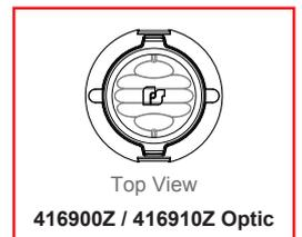
**NOTE:** For best performance, be sure to keep the horizontal lines of optics parallel to the upper and bottom edges of Federal Signal's logo before installation.
