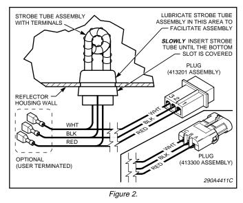
cable. Older systems will require cutting off the plug and terminating the wires with spade quick connect terminals.
