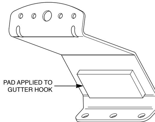
**Figure 2** Washer attached to mounting hook
