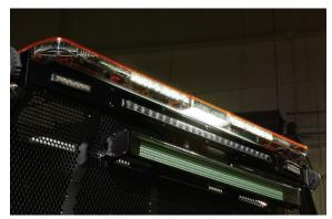
The optional bed light shines a steady work light down from the light bar onto the bed of the truck for added visibility for operators
