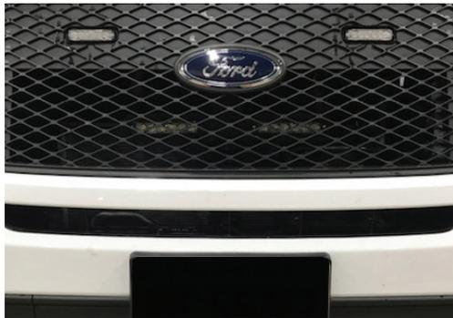
Existing IPX-GRL16 mounts (2) IPX/MPS/MPSU lights behind the upper grille
