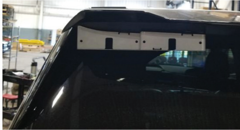
MPSM6-FPIU20RS3 mounts (2) MPS6/MPS6U lights on each side of the spoiler
