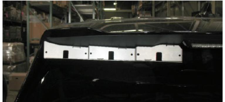
MPSM6-FPIU20RS2 mounts (3) MPS6/MPS6U on each side of the spoiler
