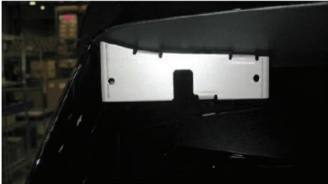
MPSM6-FPIU20RS1 mounts (1) MPS6/MPS6U on each side of the spoiler
