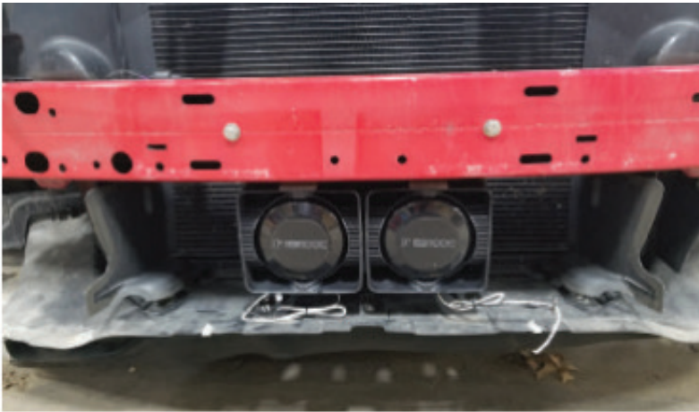
ESB2-CHGR15 installed on a 2019 Dodge Charger
