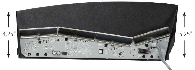
Reflector layout for Advanced Off-Axis – SIFZ models*
