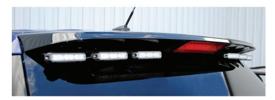
Federal Signal announces the release of a new bracket kit for the spoiler of the Ford Police Interceptor Utility. The bracket kit can be used with either the MicroPulse (MPS600) or MicroPulse Ultra (MPS600U). The kit includes brackets for mounting six light heads total — three lights on each side of the third brake light.
