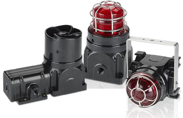
Standard models are offered in **three different mounting styles**: “Ex d” surface mount, “Ex d” with articulating U-bracket, and “Ex de” increased safety surface mount. Additionally, each signal supports a full range of voltages, including 12VDC, 120VAC, and 220-240VAC.
