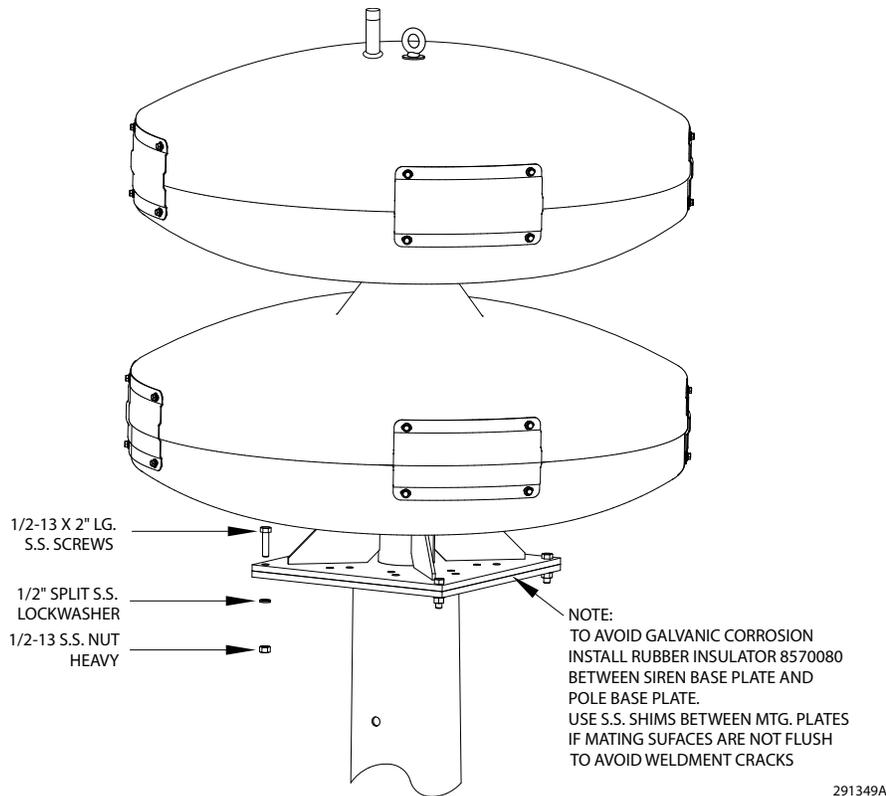
4. Attach the modulator base to the pole's top plate with rubber insulator 8570080 between them.
