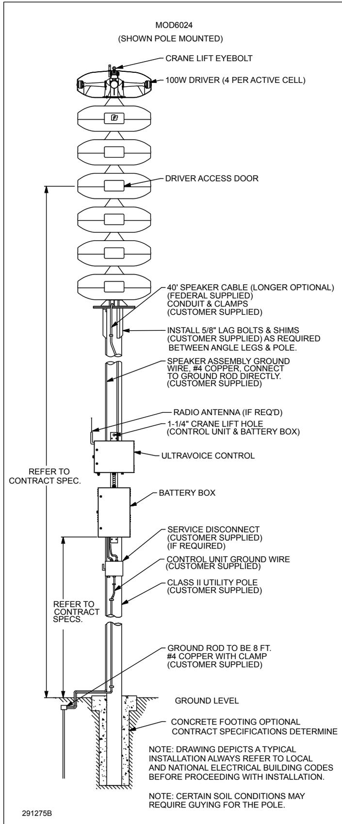
To mount the siren on the Class 2 utility pole using the three-foot-long angle iron legs:
